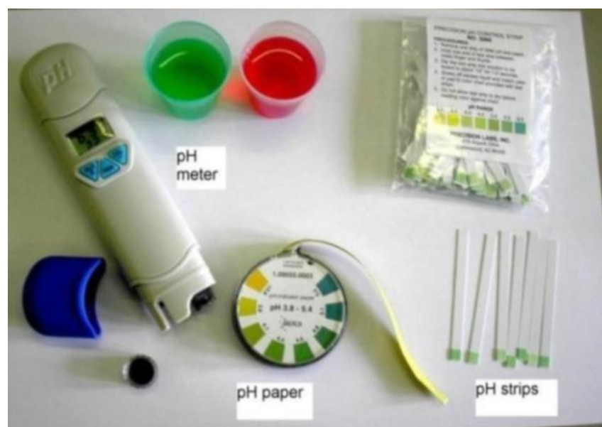
Figure 1: Equipment needed for measuring pH values
