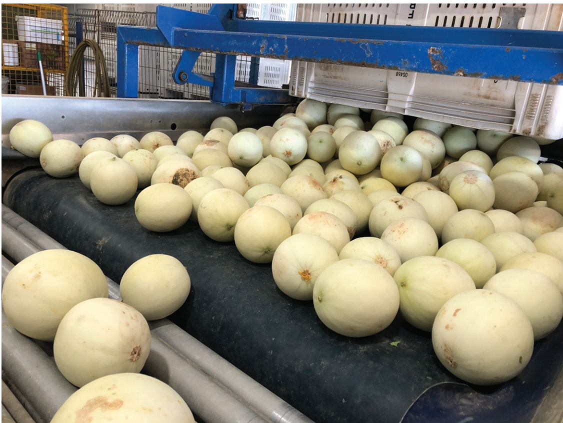
Figure 20. Dry dumping: the fruit is placed onto conveyor belts where it moves on to be rinsed, washed and sprayed with sanitisers.
