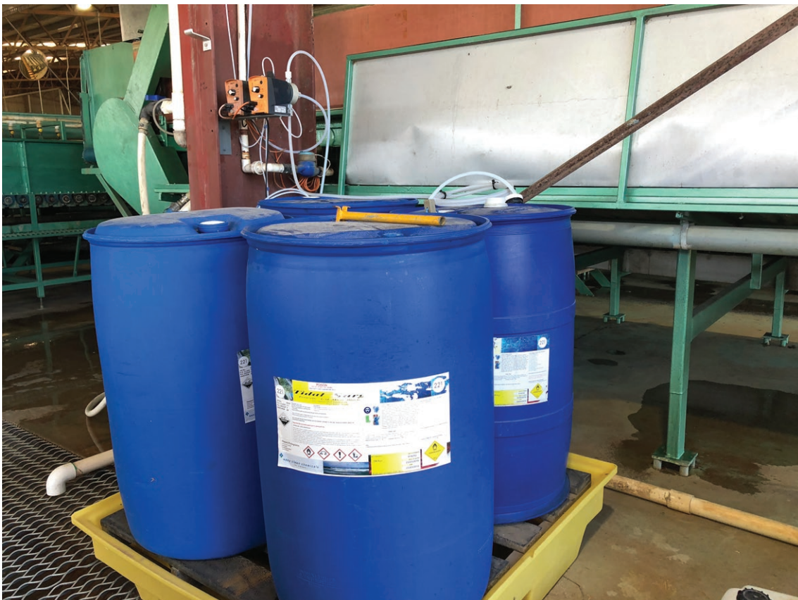
Figure 37. Peracetic acid (PAA) is being dosed into the postharvest wash water in a melon packhouse.
