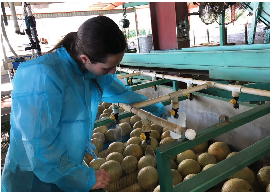
Figure 29. Wash water sampling and monitoring.
