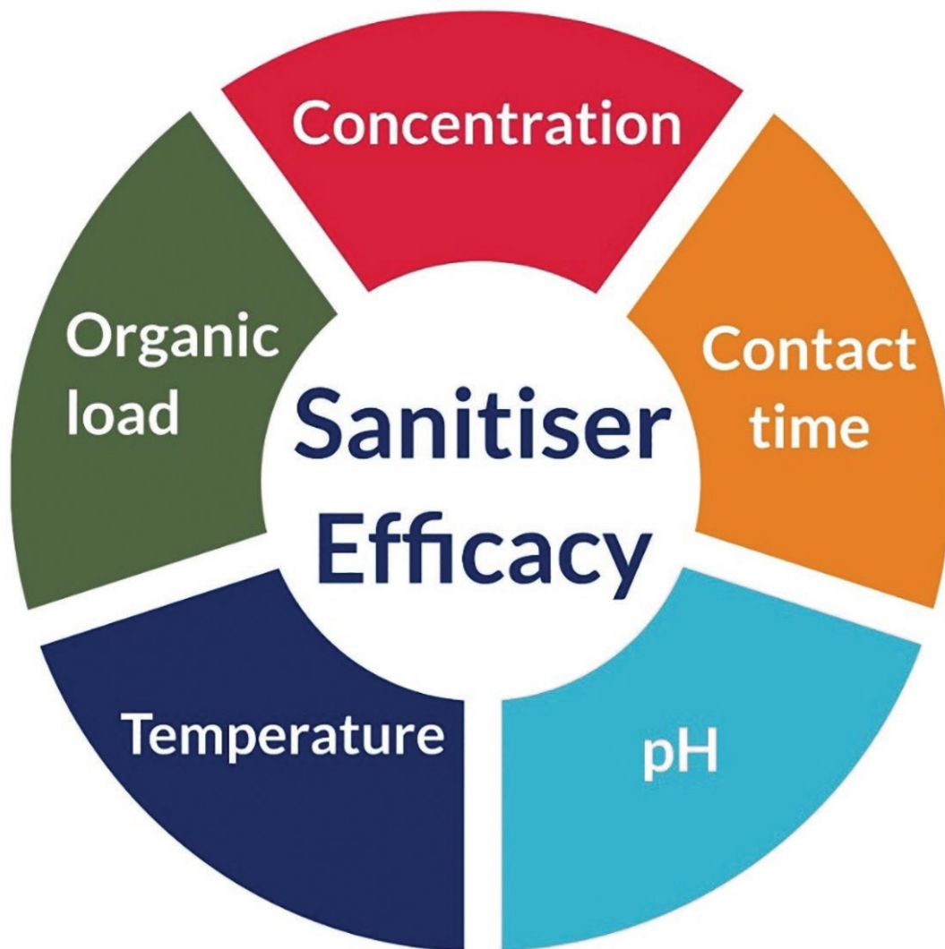
Figure 27. Sanitiser efficacy is influenced by a number of factors such as concentration, contact and exposure time, pH, temperature, water quality and organic load in the water.
